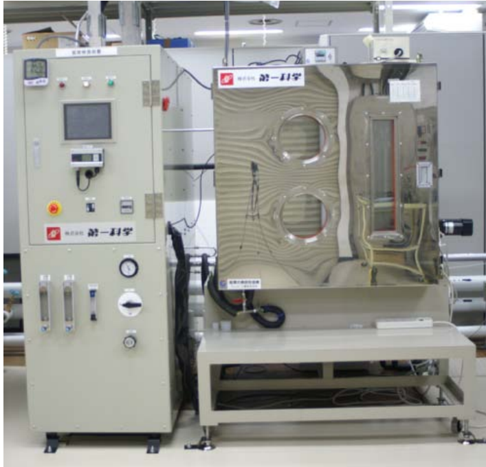
Humidity type Manufacturer: DaiichiKagaku. Inc(Japan) Model: DHHG-005-AP Range: 15% to 95%
