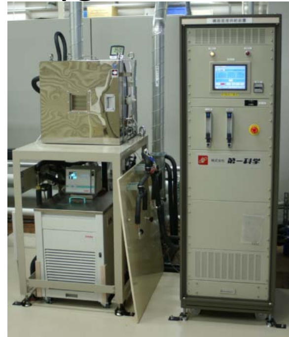
Humidity and temperature type Manufacturer: DaiichiKagaku. Inc(Japan) Model: DHHG-003-AP Range: Humidity: 10% to 95% Temperature: -10°C to +50°C
